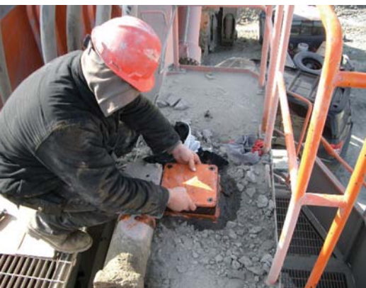
Action to reduce contamination of a Hitachi EX2500 excavator involved installing gaskets when none had been originally provided, left, and providing a flow deflector to protect filter elements from high-velocity oil, which were not provided in the original housing, right.
