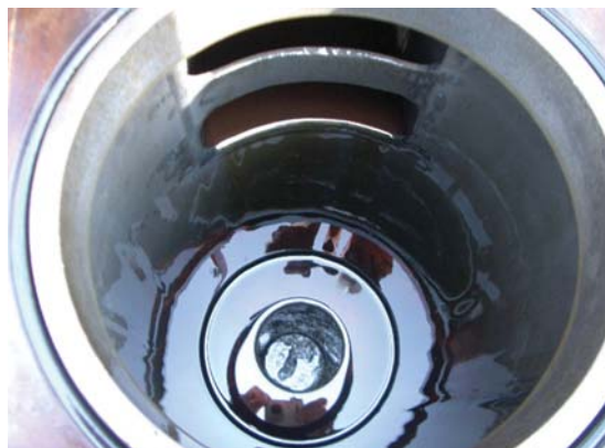
Action to reduce contamination of a Hitachi EX2500 excavator involved installing gaskets when none had been originally provided, left, and providing a flow deflector to protect filter elements from high-velocity oil, which were not provided in the original housing, right.
